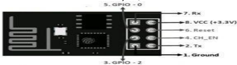
Figure 3.4: Pin Configuration of ESP8266
